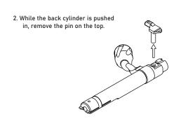
Remove the firing pin from the assembly.
