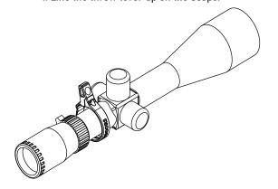
Tighten the throw lever onto the scope with the provided screw.
