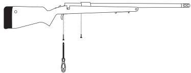
3. Replace both stock screws to fasten the gun to the new stock.
